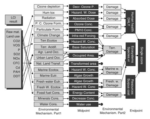
**Figure 10.4** The overall structure of ReCiPe methodology for Life Cycle Assessment Impact Assessment. Reproduced by permission of PRé Consultants B.V.
